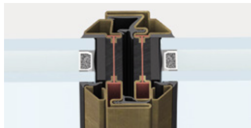
central section | frame section 62 mm
