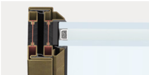
lateral point | frame section 47 mm
